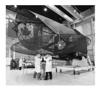
Figure 1.1: Spring back reflectors (one folded and one deployed) on MSAT-2 spacecraft. Courtesy of Canadian Space Agency.
